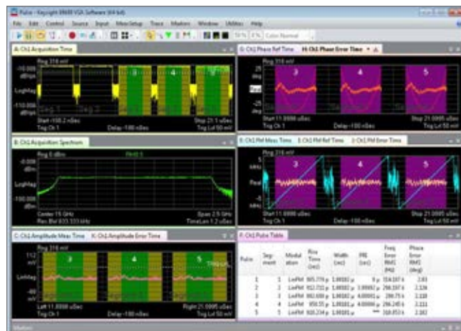
Figure 4 | Pulse-analysis software calculations based on measurements taken on oscilloscope segmented memory.
