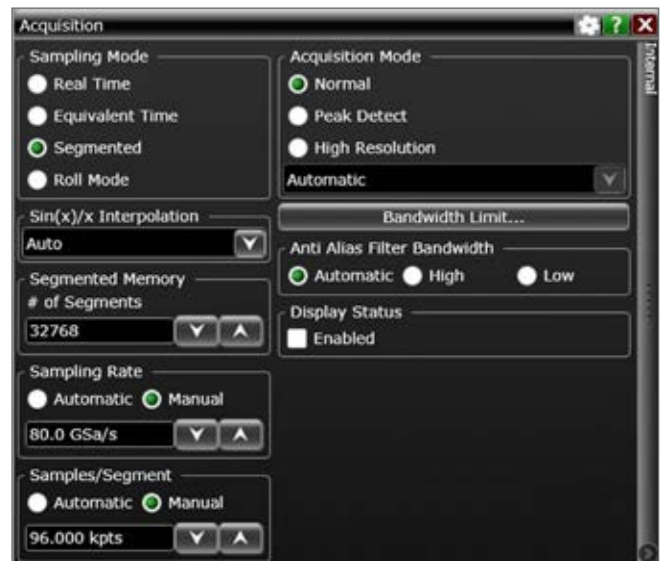
Figure 2 | Segmented memory setup to choose 1.2 usec wide segments for 1 usec wide pulse capture.
