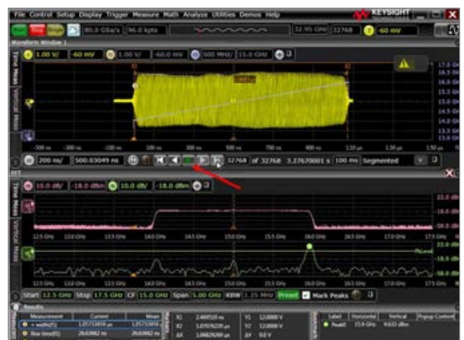
Figure 3 | 33 GHz oscilloscope segmented memory capture of 32k pulses into 32k segments, 1.2 usec per segment.
